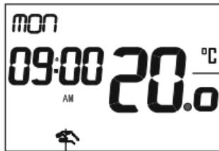
The new set temperature will flash while the change is being made
