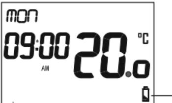
Battery low indicator will appear when the batteries are low.
