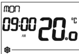
Frost symbol will continuously flash when frost protection mode is active.
